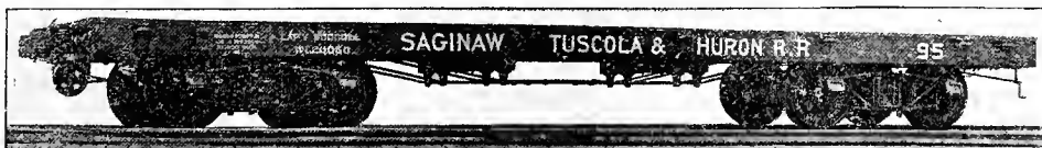
Fig. 16. FLAT CAR. SAGINAW, TUSCOLA & HURON RAILROAD. Length, 36 ft. Capacity, 60,000 lbs. Weight, 20,050 lbs. Equipped with Pull up Brake, Aldrich Brake Wheel and Swing Motion Diamond Trucks.
